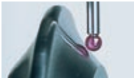
CBN-grinding tool reworking incl. stripping and replating
