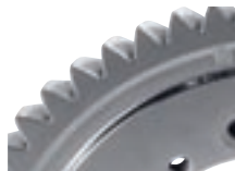
Rolling tools to remove secondary burrs and smoothen tooth flanks
