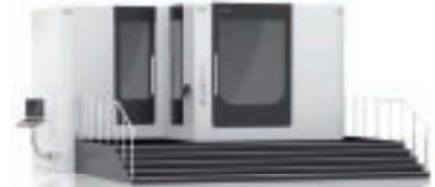
HG 2400 Ø 2,400 mm m_n 35.0 / 40.0** mm Axial travel 950mm
