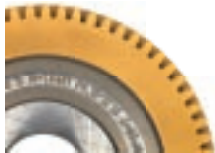
Rolling gears to check noise and improve surface finish
